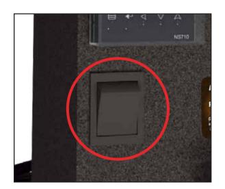
Set power switch to the "on" position. You will notice on your control screen there are two rows of digits. The top is the current temperature of the heat plates. The bottom is the set temperature. The mini comes preset at 200 degrees Fahrenheit and will take approximately 5-7 minutes to reach set temperature depending on your location.
