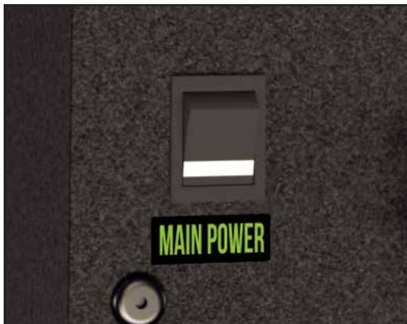
Set power switch to the "on" position. You will notice on your control screen there are two rows of digits. The top is the current temperature of the heat plates. The bottom is the set temperature. The OG comes preset at 200 degrees Fahrenheit and will take approximately 10-12 minutes to reach set temperature depending on your location.
