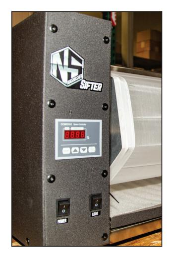
Thank you for your purchase of the NS Sifter. Each unit is hand built in Corona, CA., with precision and quality that the Nugsmasher brand is known for. The exterior of machine is made from solid steel which is powder coated for long term use and cleanliness. The interior skin of the NS Sifter is fabricated using food grade stainless steel and will provide for an excellent non stick clean surface.
