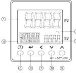
1 Pvdisplay window (displays measurements, parameter names, and so on)
